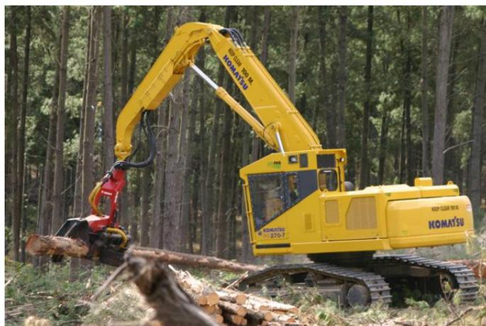
Figure 1 An operative protective structure that is being used for forestry applications.
